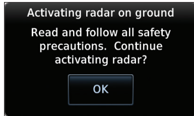
Figure 12-61 Caution for Radar Activation Confirmation
